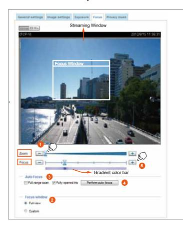
Below is the procedure to perform the automated Zoom and Focus function:
